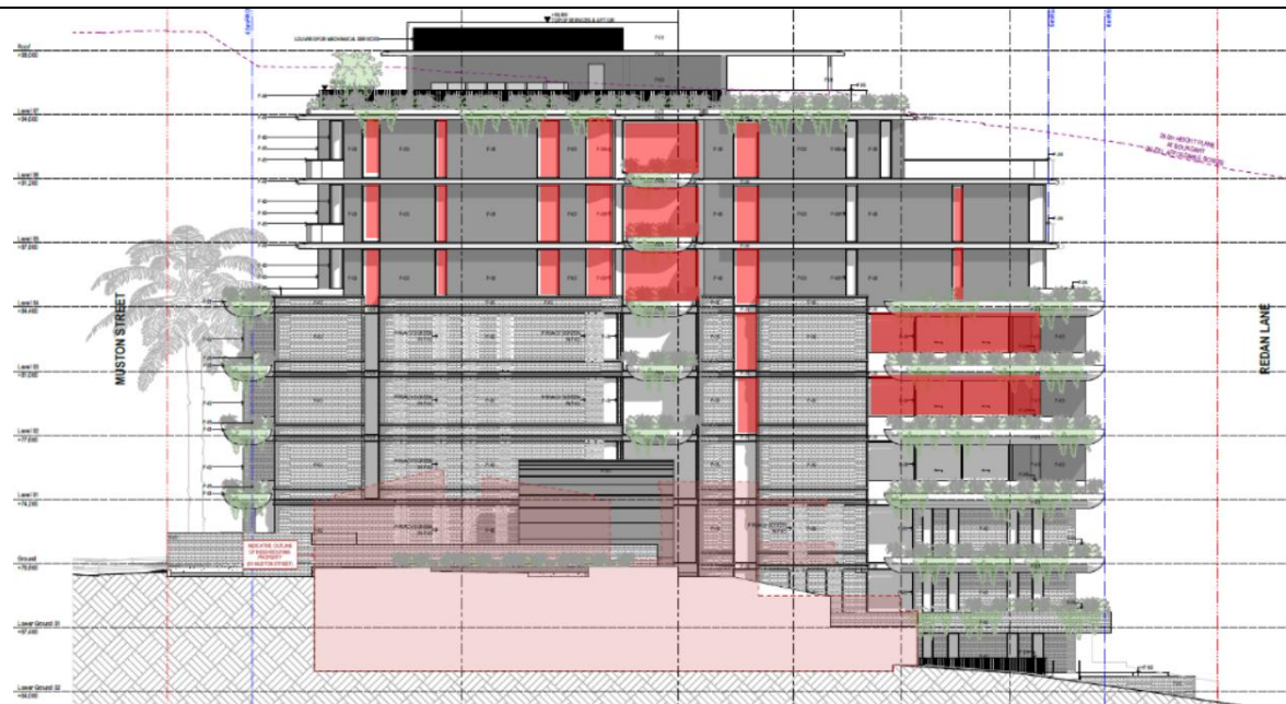
Extract from South Elevation Drawing A-210-020 with red mark-up of windows not meeting ADG requirements (Source: Studio Johnston)
