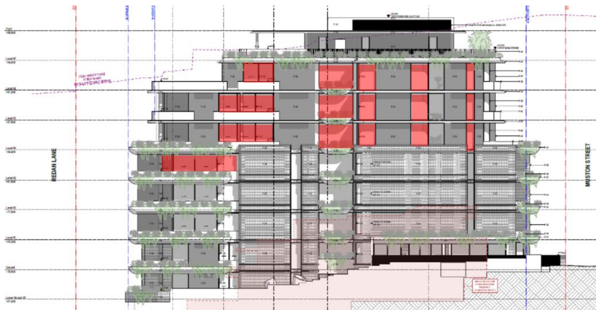
Extract from North Elevation Drawing A-210-010 with red mark-up of windows not meeting ADG requirements (Source: Studio Johnston)
